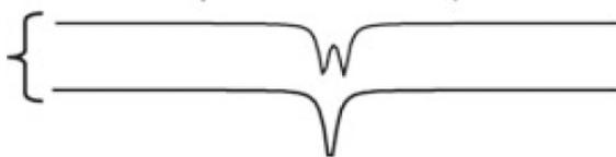
*The standard pattern of a steel in which ferrite and austenite phases are present. The  $^{57}\text{Fe}$  Mössbauer spectrum of the sample is a complex spectrum that is a sum of subspectra. The subspectra of the ferromagnetic ferrite with bcc lattice and the paramagnetic austenite with fcc lattice are also superimposed from elementary patterns because of the effect of alloying elements, although the Fe atoms can only occupy one single crystallographic site in each phase.*
